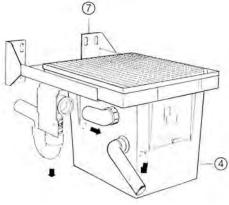
3.1.6 Push the plaster trap 4 into support W (7).
