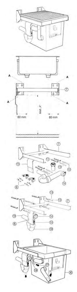
3.1.5 Insert the in-flow cover ③ in the plaster trap ④ and place the splash-guard grid ② in the in- flow cover ③.
