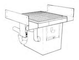
3.4.1 Measure and mark the 8 mounting points **C**. Measure "X" for floor-mounted cupboards 83 TL, 83 TR = 202.5 mm
