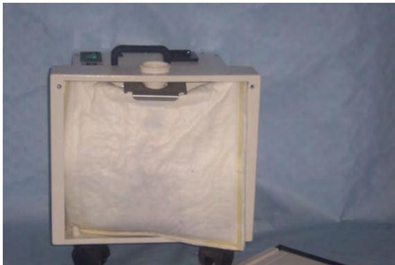
Fig.1/2 Exchange of the filterbag
