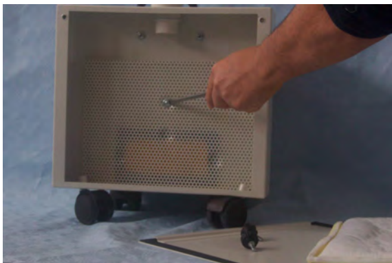
Fig.3/4 Exchange of the motorprotectfilter
